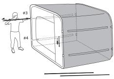
Hold the frame with one hand and the bottom horizontal bar with the other hand and rotate the tent
